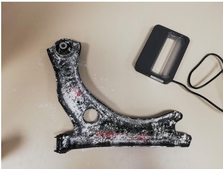
Figure 36: Control arm ready for scanning.
