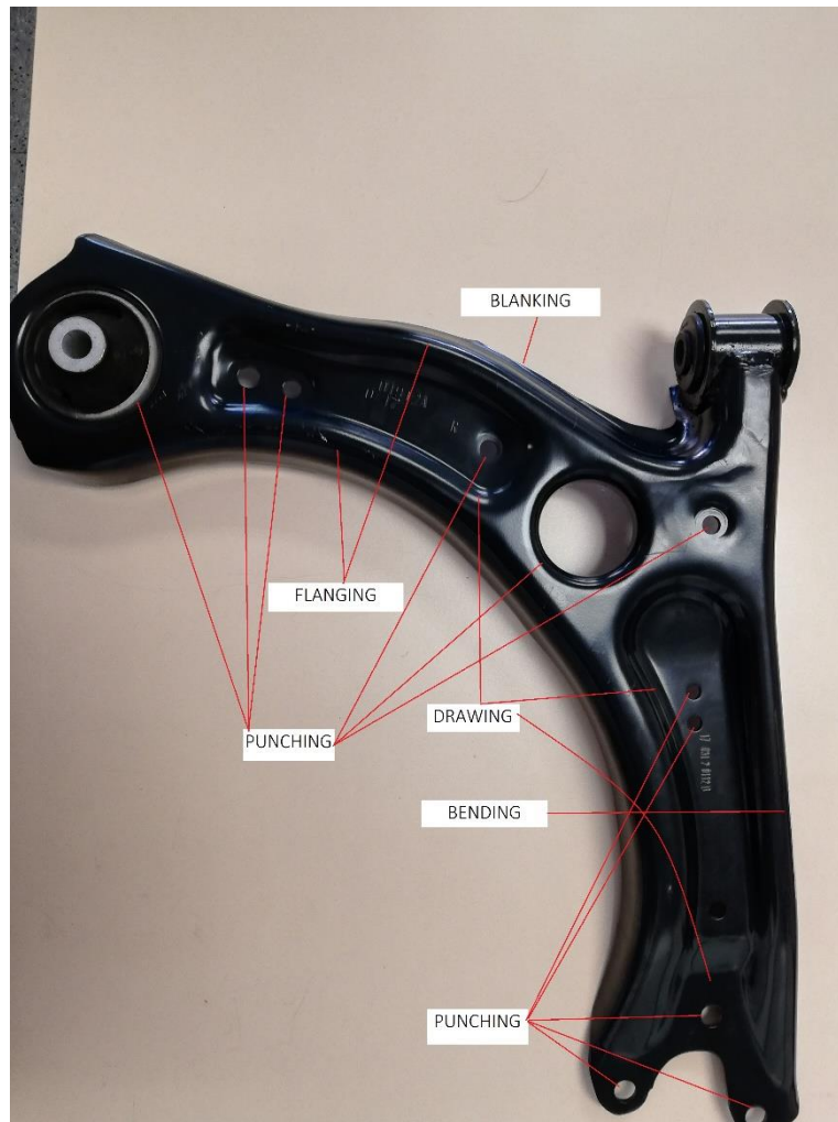
Figure 2: Operations performed to obtain a control arm.
