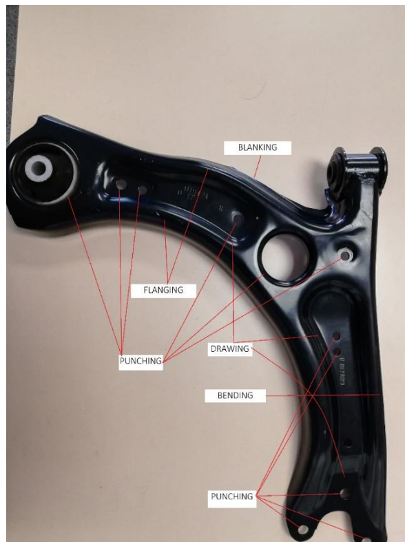
Figure 2 (Rep.): Operations performed to obtain a control arm.
