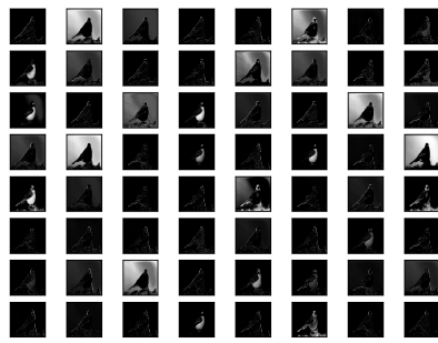
(a) Visualization of the feature maps extracted from the first Convolutional Layer in the VGG-16 Model [1]
