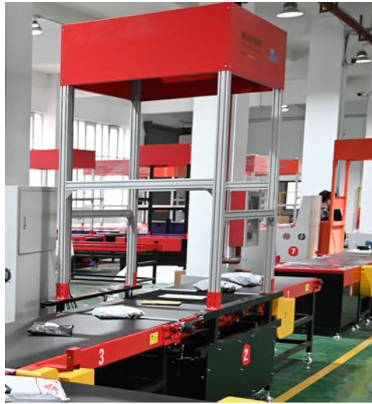
Figure 6.1: Automatic weighing and scanning machine. [33]
