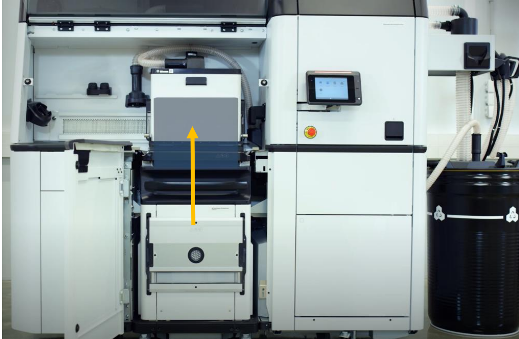
Figure 4.6: HP MJF Extract from BU to NCU operation. [9]
