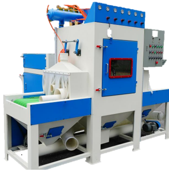
Figure 6.2: Automatic cleaning machine with conveyor. [34]
