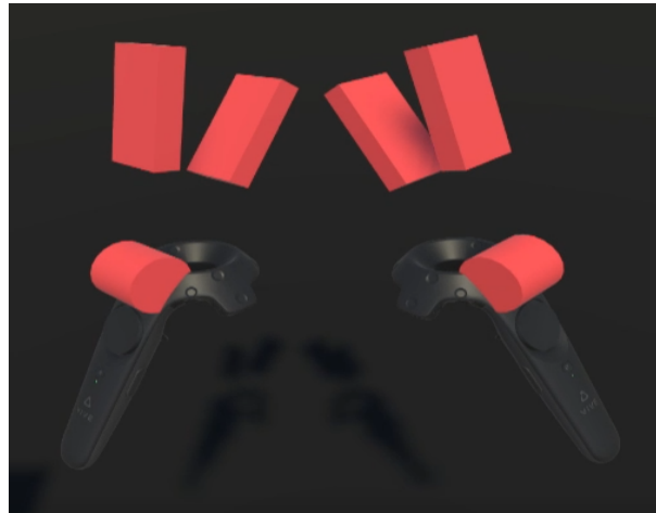
Figure 49: Model of a robot's claw attached to HTC's controllers. The claw was created with one fixed cylinder, one fixed box, and one moving box.
