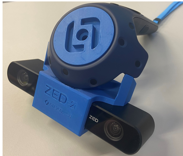
Figure 53: Accessory for ZED 2i and HTC controller attachment.
