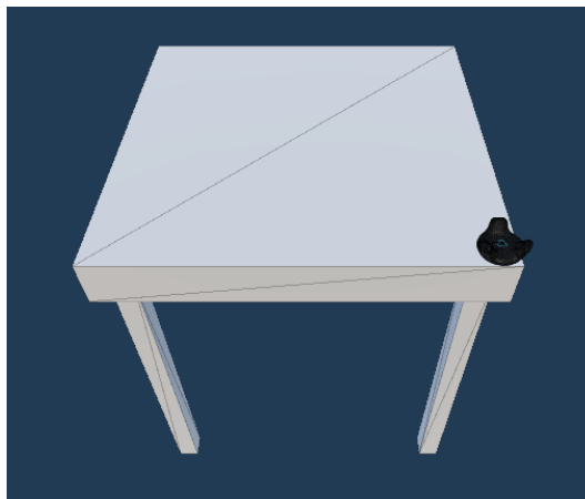
Figure 55: View of virtual table prefab. Notice how the prefab has a virtual HTC tracker on its bottom right corner. This virtual tracker has a real counterpart located within the real world, allowing a precise calibration for the virtual scene.
