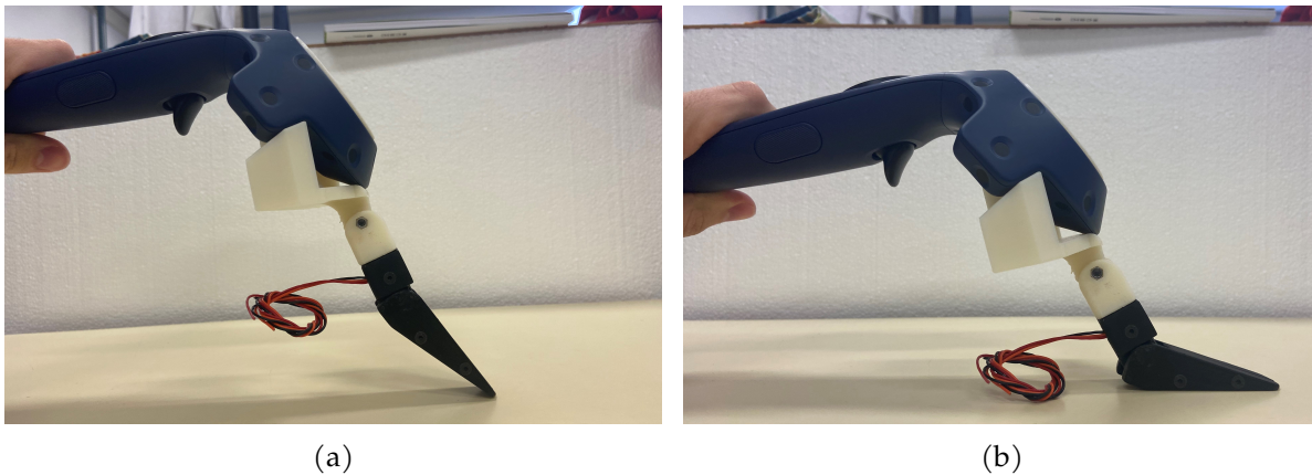
Figure 64: 3D printed gripper accessory for HTC controllers. Notice how, when pressure is applied, the external part of the gripper folds in order to properly grasp garments.
