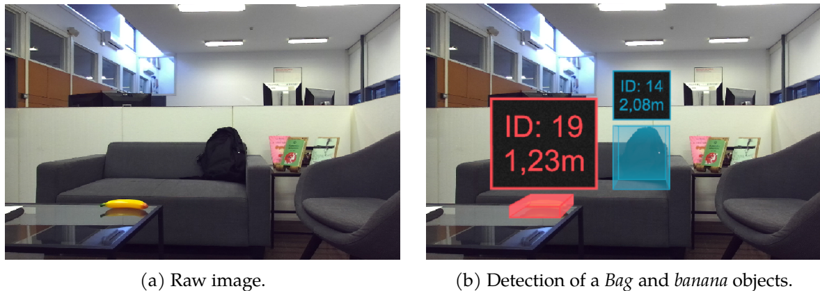
Figure 39: ZED's object detection implementation into Unity . When a object is detected, ZED's SDK uses depth information to estimate the distance between the camera and the object. Also, the software identifies each object with an ID to be able to track them.
