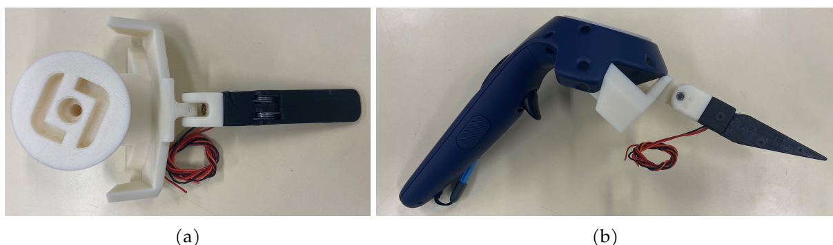
Figure 63: 3D printed gripper accessory for HTC controllers.
