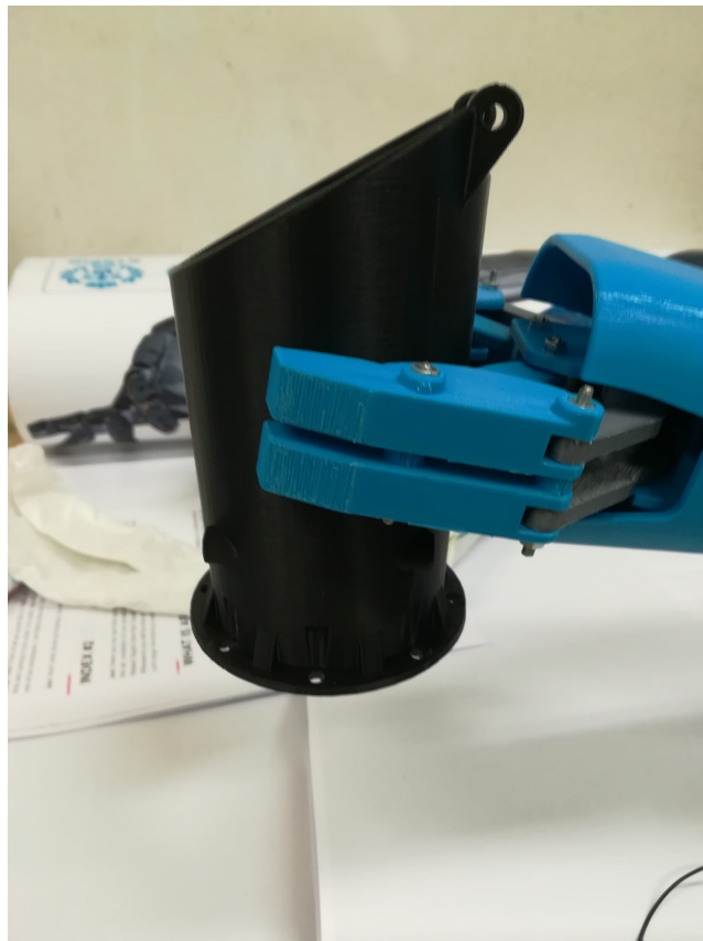
Figure 2.4: Lift capacity testing of Andromeda at ARM2u's office, ETSEIB. Source: self.
