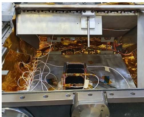
Figure 6: LEDSAT inside the TVAC chamber. Upon changes on the environmental requirements from the launch authority, it was found necessary to perform additional tests on the CubeSat. To this end, the team travelled to the Astrofein facilities in Berlin to perform a shock test on the payload EM (Engineering Model) in May 2021 and to the CubeSat Support Facility (CSF) in ESEC Galaxia in June 2021 to perform new vibration and thermal-vacuum testing on the PFM (Proto-Flight Model), see Figure 7.
