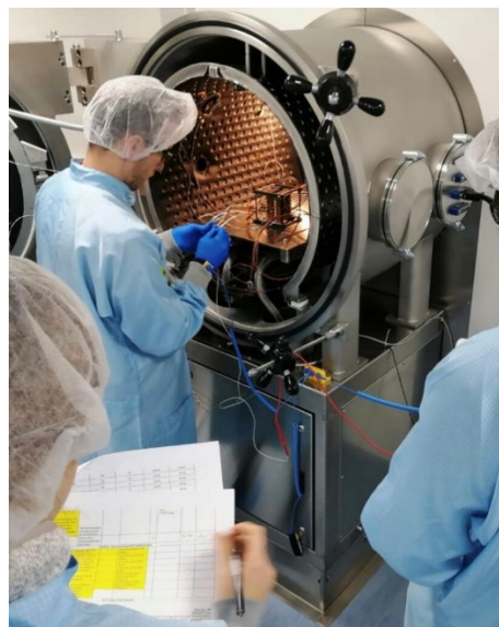
Figure 5: Students performing the TVAC testing on the payload at the CSF.
