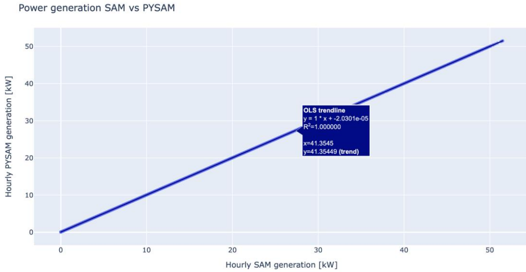
Figure 60 Linear regression of power generation hourly values from SAM and from the tool for the estimation of solar PV generation.
