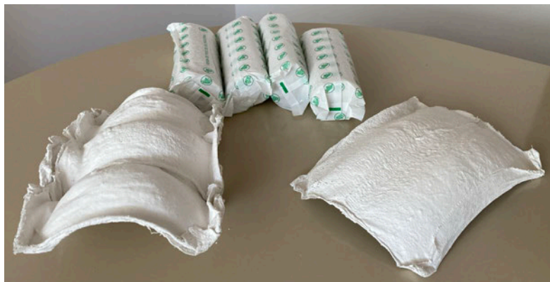
Figure 7. Kit to explore surface hanging models with gypsum.
