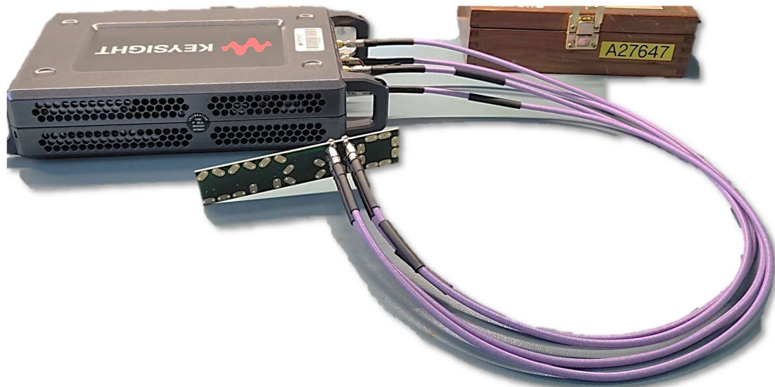
Figure 7: Keysight 53GHz 4-Port VNA connected to a test board
