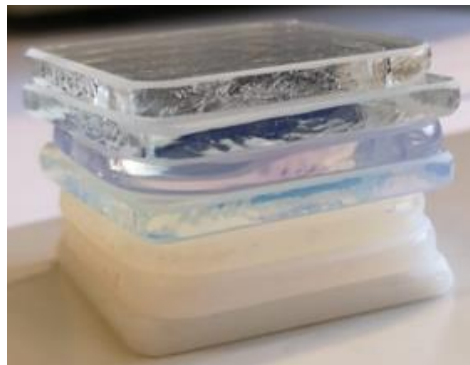
Figure 1. Silica Glass stack with changing scattering depending on the size of the microstructure. Average particle size increases from top to bottom.
