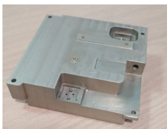
Figure 7. Post-machined propulsion housing with surface treatment for corrosion protection
