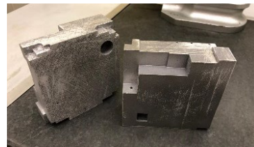
Figure 5. Printed parts, with support structures removed
