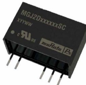
Figure 72: Isolated DCDC Converter MGJ2D series from Murata
