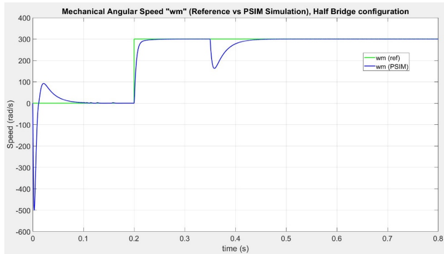
Figure 48: Mechanical Angular Speed " \omega_m " (Reference vs PSIM simulation) in a Half bridge configuration
