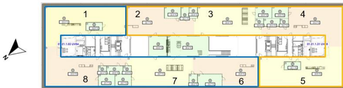
Figure 5.3.2.1: Example off floor plan with climatic zones for NOB's level 2
