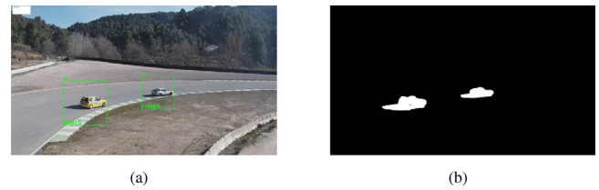
Fig. 7. (a) Two cars in the racetrack with bounding boxes around them, obtained after performing background subtraction on the frame. (b) Thanks to a static background, the task of separating moving objects from the background is largely simplified. The regions of interest after applying simple computer vision techniques are much smaller than the whole FullHD frame captured by the camera lens, which allows us to focus the attention closer to the objects and increase the accuracy of the ground-truth model. In an scenario like the racetrack of the image, motion detection alone is able to filter all empty frames out and only consider those with cars and minimize the annotation costs.
