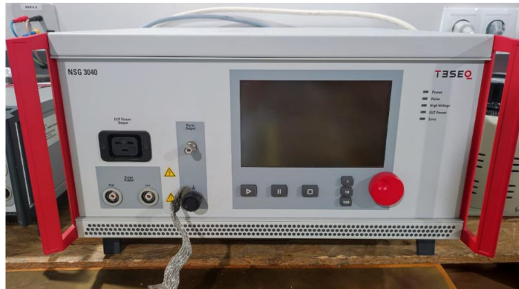
Figure 50: Teseq NSG 3040 Surge generator.
