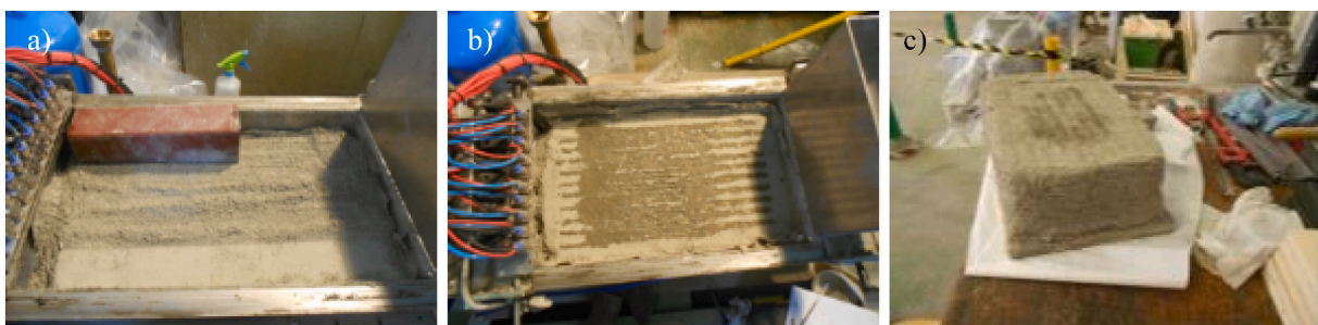
Fig. 5. Production process: a) compaction, b) penetration of the reactive agent, and c) final element.
