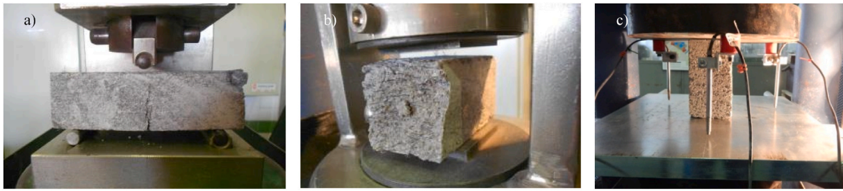
Fig. 4. a) 3-point bending test, b) compressive test and c) setup for assessment of elastic modulus.
