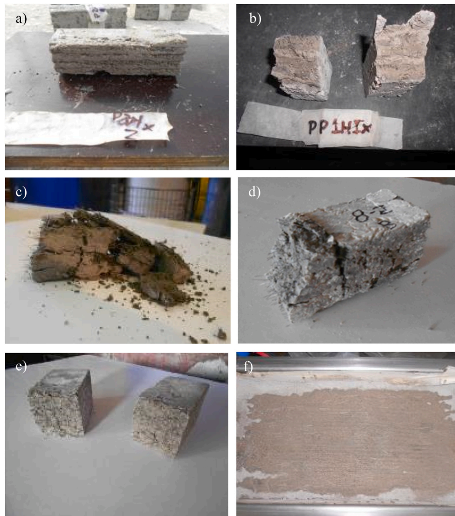
Fig. 6. a) Layers in the cut surface of the beam, b) cross-section of a beam showing non-uniform hydration, c) beam from batch 7-M-7-7LX, d) beam from batch 8-M-7f-7LX, e) beam from batch 10-M-5a-7LX, and f) layer with roughness to improve the bond.
