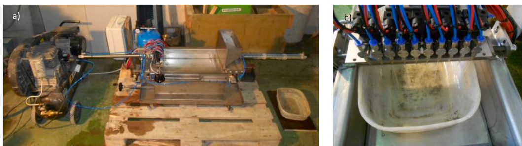
Fig. 1. a) Small-scale particle bed system and b) printer head with 10 electrovalves or injectors.
