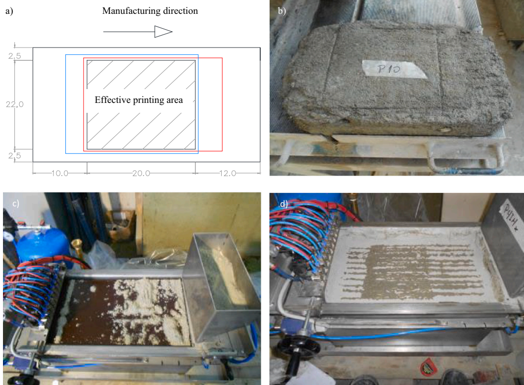
Fig. 2. a) and b) Effective surface of irrigation, c) distribution of solid components, and d) irrigated surface.
