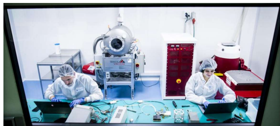
Fig. 1. UPC NanoSat Lab clean room with TVAC and shaker
