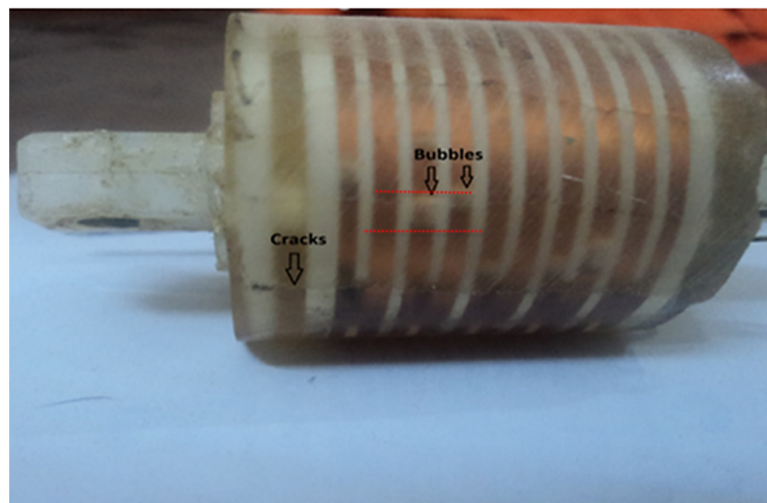
Figure 1. The bubble and cracks inside the insulation of the ignition coil.
