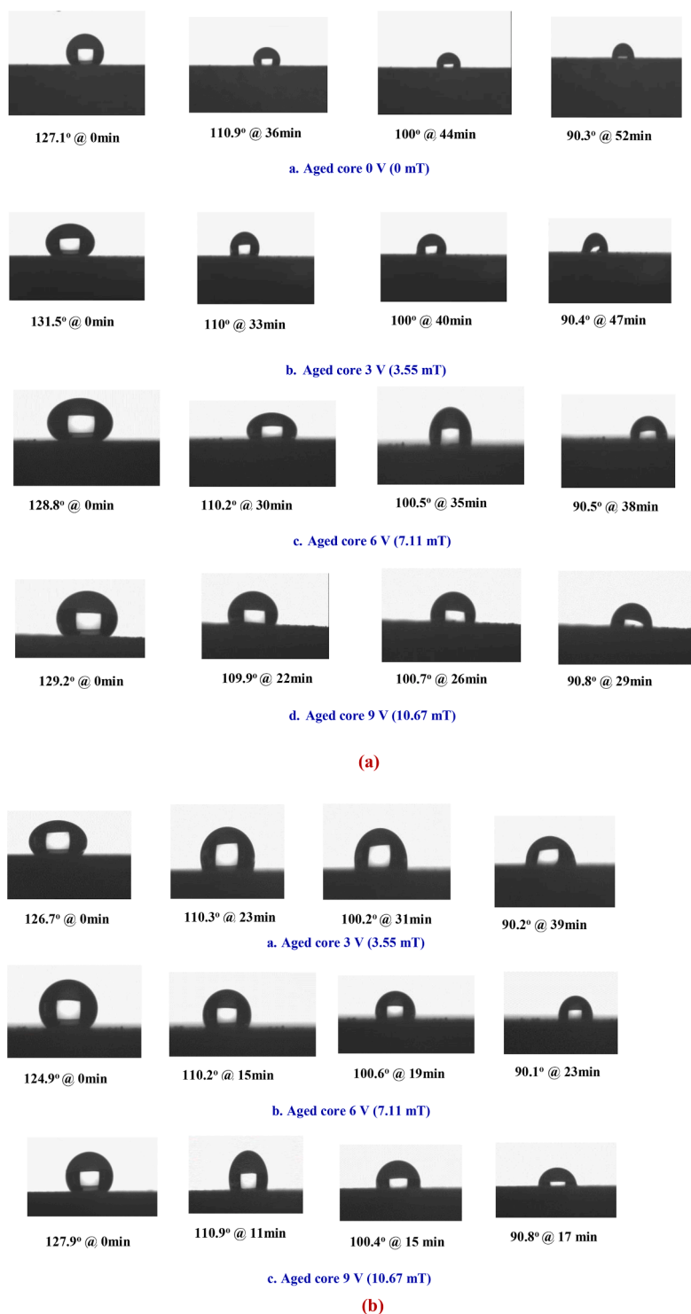
Fig. 5. Images of DW droplets the in presence of EH (a) 1st hour, (b) 2nd hour of the test.
