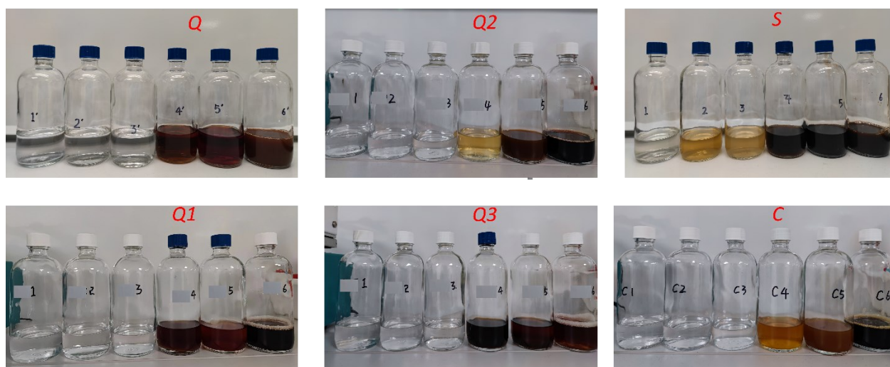
Figure 19: Sequential ASE extracts of six crude tannins. Each tannin sample was extracted with the following solvents, from left to right, hexane, MTBE, DCM, acetone, EtOH, and H 2 O.
