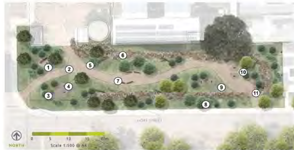
Figure 4. WGV sump park landscape plan. (Key: 1. Informal nature play with climbing logs; 2. Pathways made from crushed recycled rubble; 3. Gross pollutant traps; 4, 9, & 10. Bubble-up pits from underground cells; 5. Air-vent for underground cells; 6. Limestone boulders; 7. Log seats; 8. Planted street verge; 11. Steps.) Credit: JBA.
