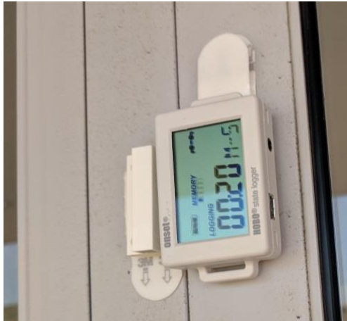
Figure 3-6 HOBO state logger installed on a sliding door in closed position
