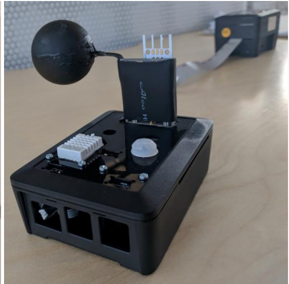
Figure 3-4 Close-up of the Raspberry Pi IEQ monitoring device.
