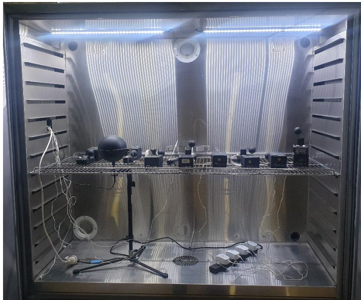
Figure 3-5 Raspberry Pi IEQ monitoring devices and the reference temperature sensors within the climate chamber prior to calibration.
