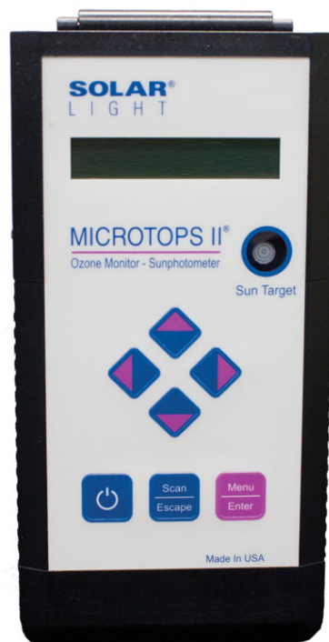
Figure 8: Solar Lights Hand-held Model 540 Microtops II Sun photometer that is used within this study. The instrument must be directed at the sun whilst there is no cloud coverage, and the Sun Target assists the user to ensure that the instrument is within the field of view (Solar Light, 2020).
