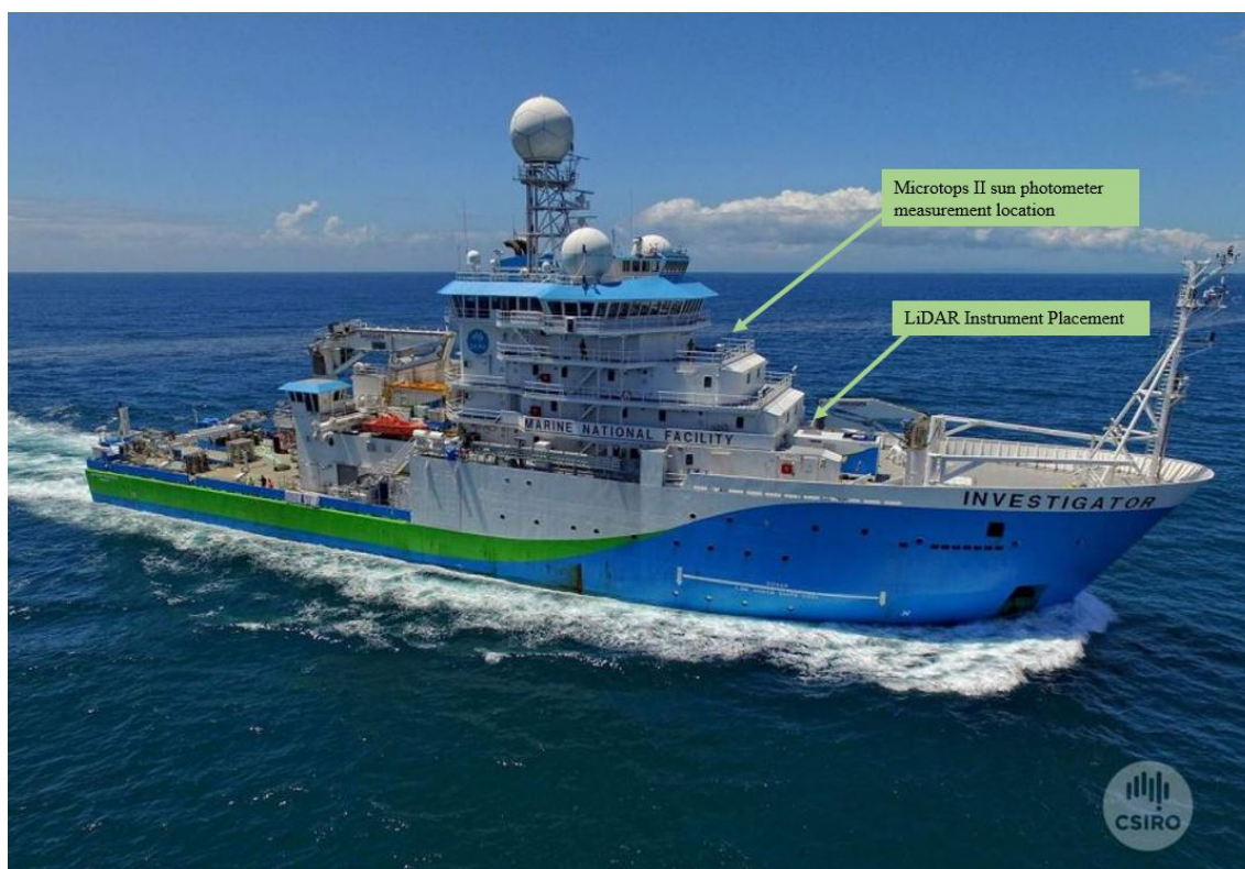
Figure 6: The RV Investigator with the sampling location the Microtops II sun photometer was used and the LiDAR instrument placement during the CAPRICORN II campaign (CSIRO, 2020b).
