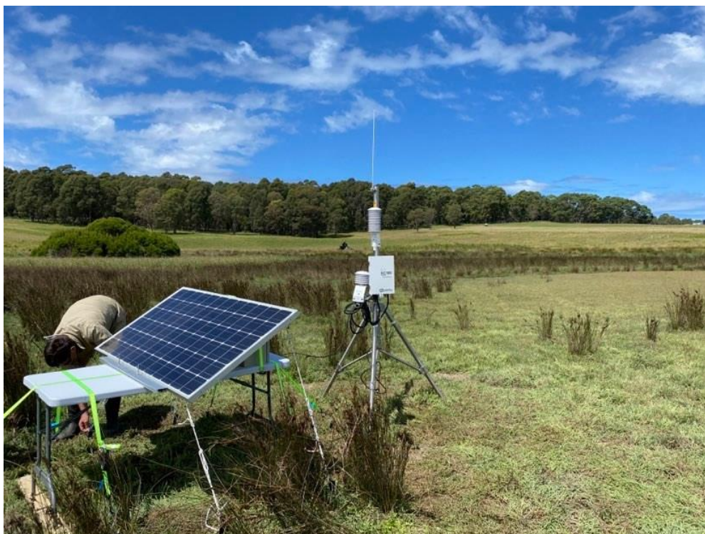
Figure 5.1: Photograph of the initial eddy co-variance tower set up. The table in the lower-left corner holds the solar panel and battery use to power the tower.
