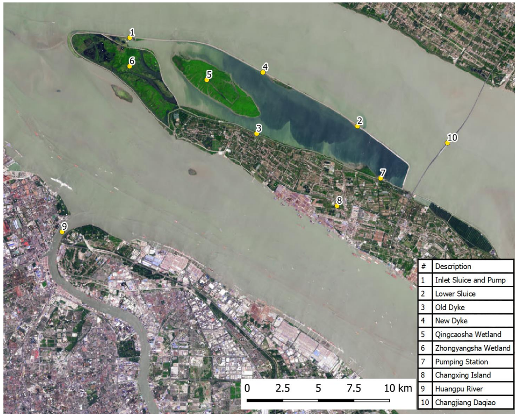
Figure 4-3: The Qingcaosha Reservoir. Aerial photo from NASA Earth Observatory (2017). Key locations from Sogreah Consultants (2008)
