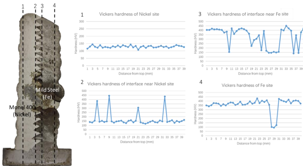
Figure 4.3.5 (3). Hardness distribution from the bottom to the top in the cross-section of Wall 3 (LCS/M400)
