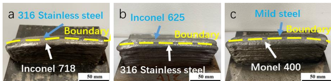
Figure 4.3.1. Three thin wall samples (a) Inconel 718 (IN718)-stainless steel 316 (SS316), (b) Inconel 625 (IN625)-stainless steel 316 (SS316), (c) Monel 400 (M400)-Mild steel (LCS)
