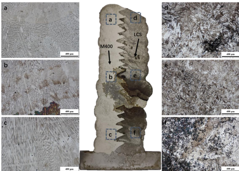
Figure 4.3.3 (3). The representative microstructure in both LCS and M400 sides of Wall 3
