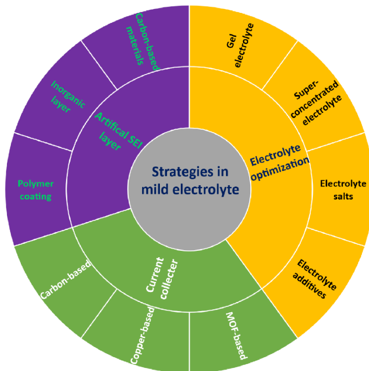
Figure 2.12 Summary of the strategies for addressing the problematic issues for Zn electrode in mild electrolyte.
