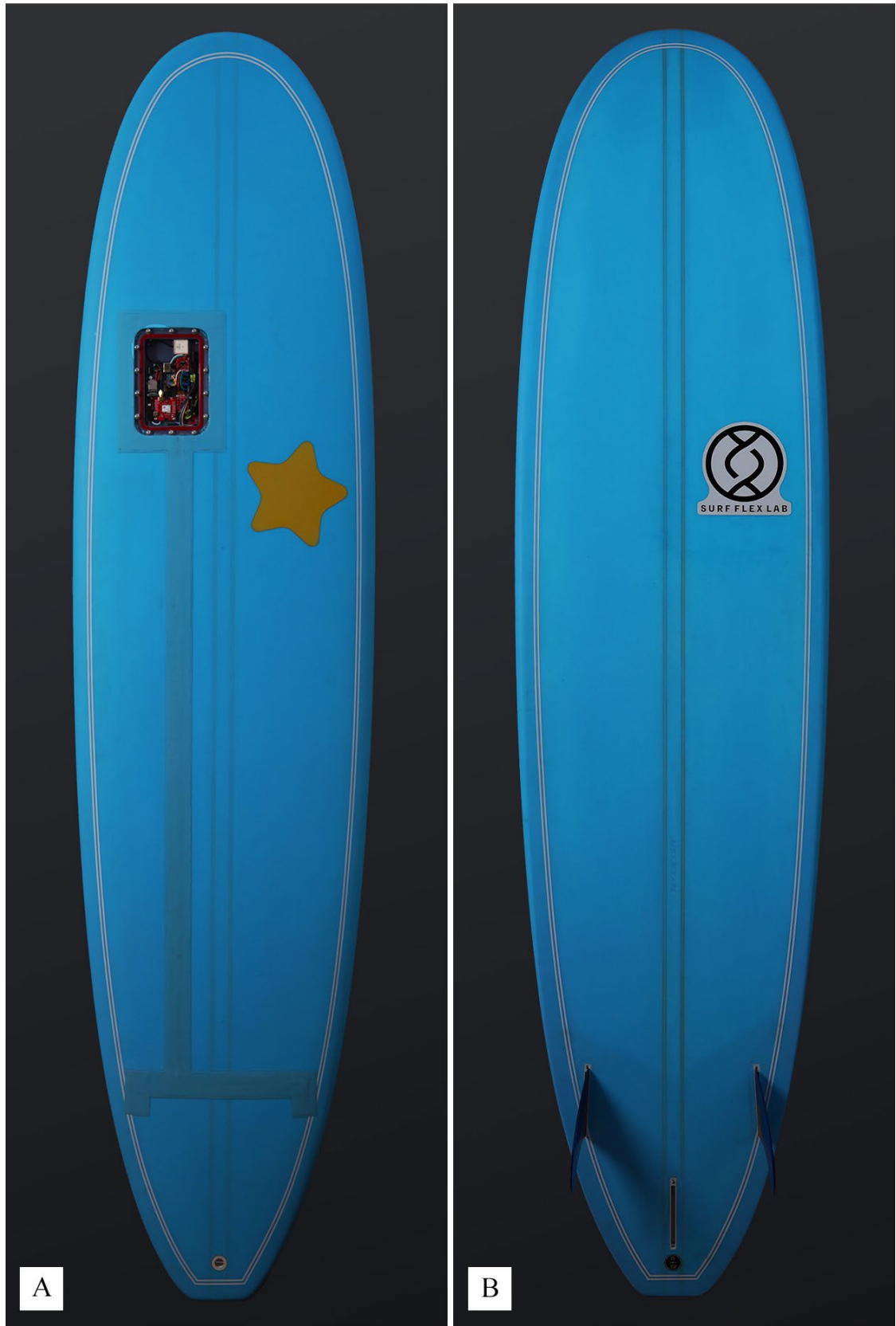
Figure 4.12: Photography of a surfboard, and instrumented fins prototypes with inbuilt data telemetry unit. A) top view. B) bottom view.
