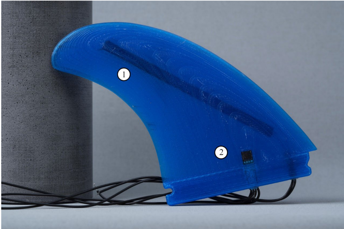
Figure 4.3: Image of the working prototype of an instrumented fin with visible 3D printed flex sensor (1), and commercial Wheatstone bridge (2).
