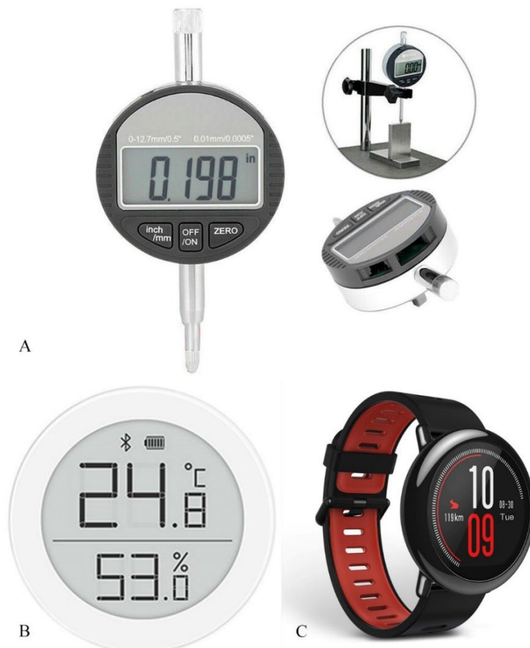
Figure 2.5: A) picture of a dial indicator used in pandemic tool [58]. B) picture of a Mijia temperature and humidity meter [59]. C) picture of a Xiaomi Amazfit Pace A1612 smartwatch [60].
