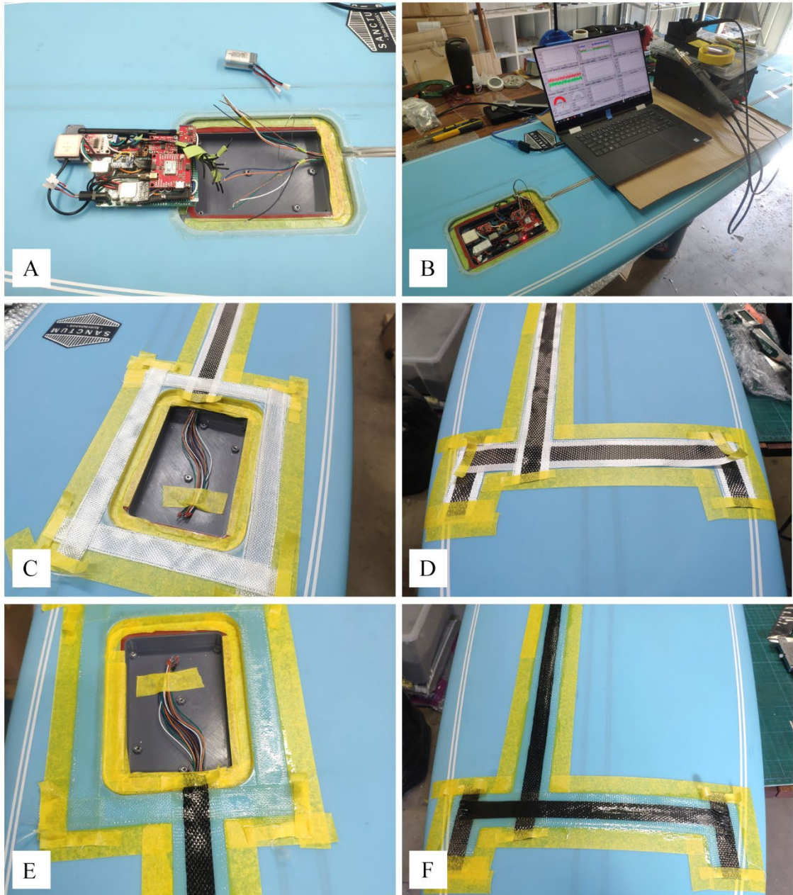
Figure 4.11: Pictures of subsequent stages of an instrumented surfboard prototype development. Letters A-F indicate: connecting electronics (A), testing telemetry system (B), custom fit of fibreglass and carbon fibre tapes (C, D), glueing fibre tapes with epoxy resin (E, F), respectively.
