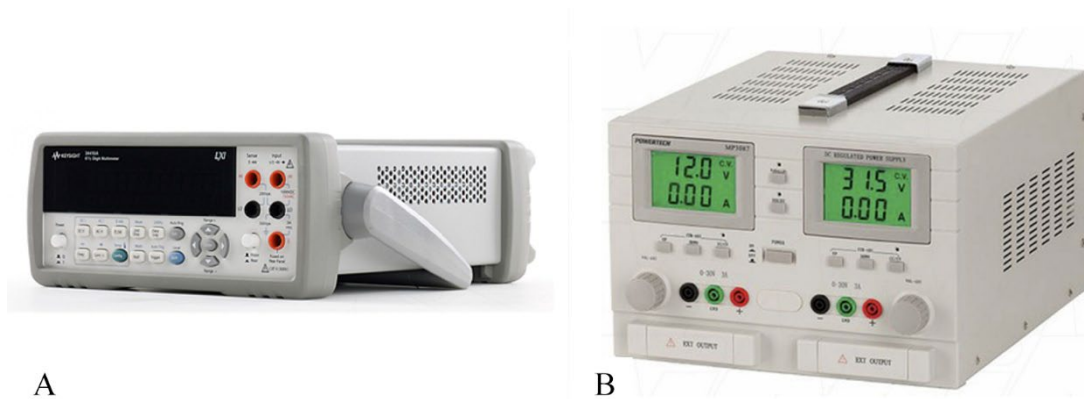
Figure 2.27: A) picture of a Agilent 34410A digital multimeter [76]. B) picture of a Powertech MP-3087 power supply [77].
