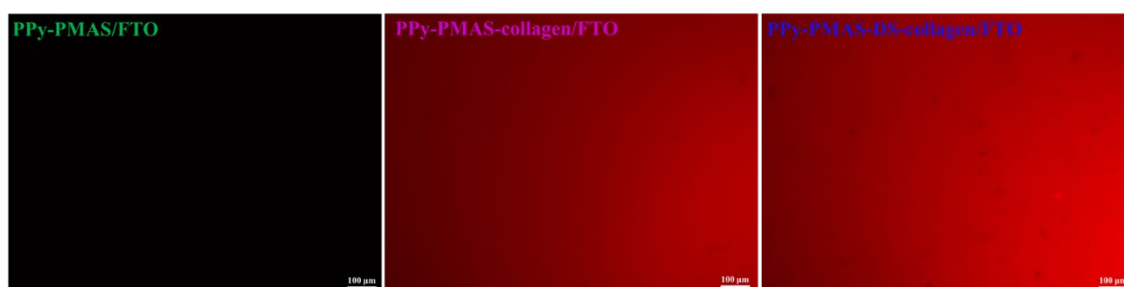
Figure 4.3 Fluorescent labelling to identify successful collagen incorporation within PPy matrixes. Images of the surface morphologies of fluorescently labelled PPy-
