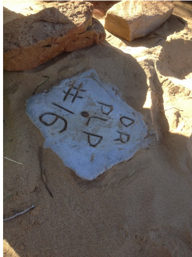
Figure 5.4. Monumentation of survey mark made by excavating into sediment, to a spade's depth and setting a 100 mm nail into the centre of a block of levelled concrete. Each concrete marker was engraved with the original project name 'DRPLP' and allocated a unique ID. DRPLP16 is depicted. Five survey marks were setup at UPK 7 in this way in August 2014. Due to Baboon disturbance, DRPLP14 had to be removed and a new survey mark, DRPLP19, set up close to where DRPLP14 was originally installed. DRPLP19 is a 0.5 m length rebar (10 mm diameter) that was hammered into the ground (as of 2016).
