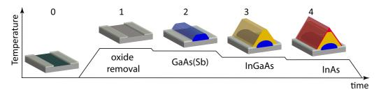
FIG. 1. Schematics of growth steps of InAs/InGaAs/GaAs(Sb) SAG nanowires on GaAs(001) substrates covered with a 10-nm thick  $SiO_2$  mask. 0. Substrate fabrication; 1. Native oxide removal; 2. GaAs(Sb), 3. InGaAs and 4. InAs layer growth. Note that the originally faceted GaAs(Sb) buffer becomes rounded after the growth of InGaAs and InAs layers on top.
