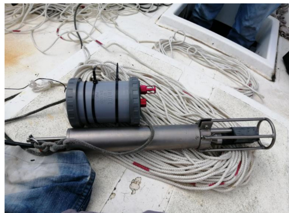
Figure 4. SPV TD aside the Sea & Sun CTD 48Mc probe; the respective lengths are approximately 20 cm and 45 cm long.
