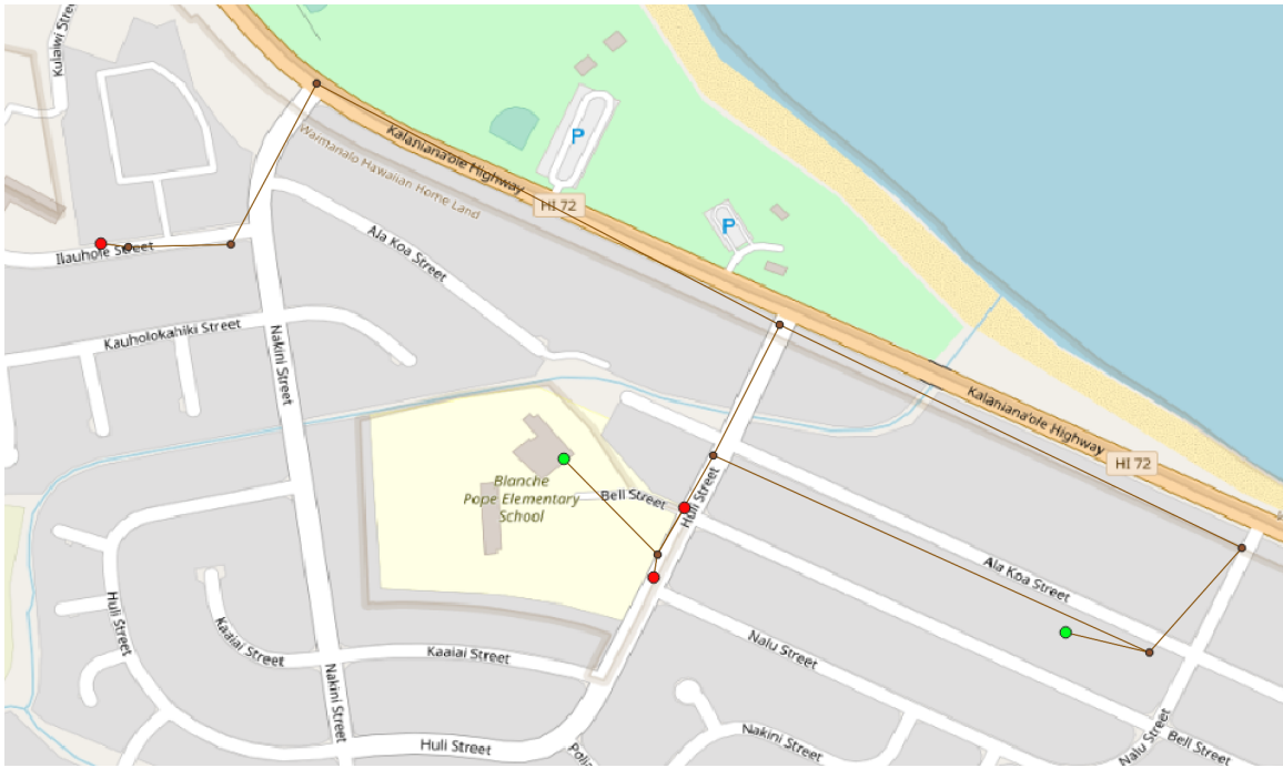
Figure 3.9. Example Model Network. Populations are indicated in green, transshipment nodes indicated in brown, PODs are indicated in red. No cost arcs connecting the populations and PODs to the network, and the road network are used as the arcs. Demand from the population centers travel via the network through transshipment nodes to the PODs.
