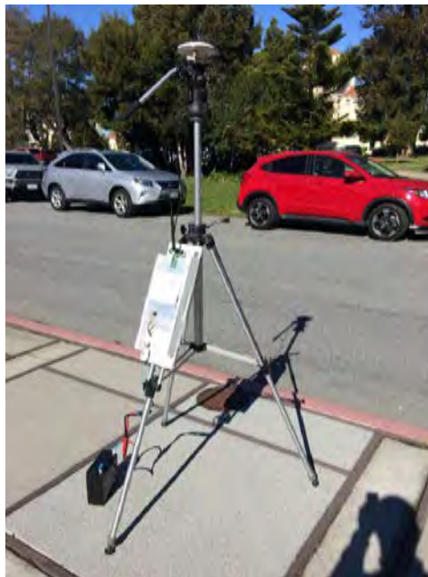
Figure 35. GPS base station enabling RTK GPS with 1 cm precision.
