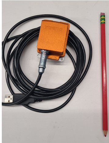
Figure 2.4. This Xsens IMU recorded inertial motion data in every set of recorded data. Pencil included for scale.
