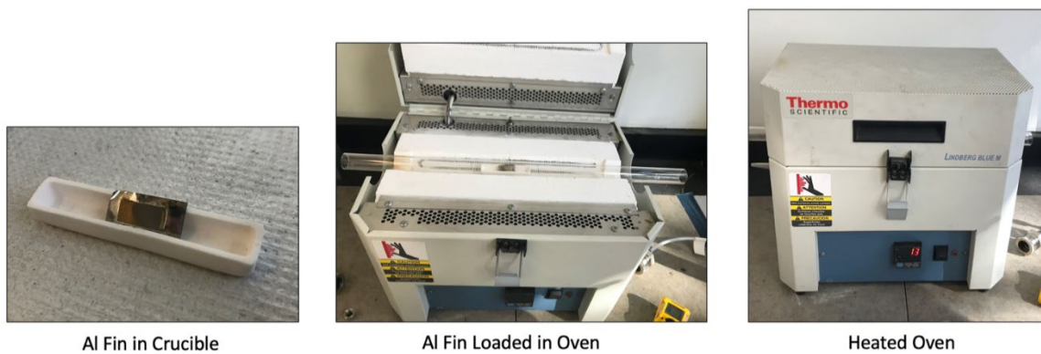
Figure 14. Annealing crucible with sample and oven
