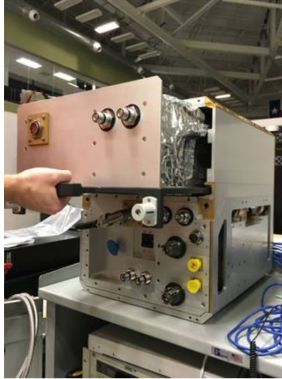
Figure 4. Removable drawer that can store up to 4.5 kg of PCM in aluminum panels. Source: [21].
