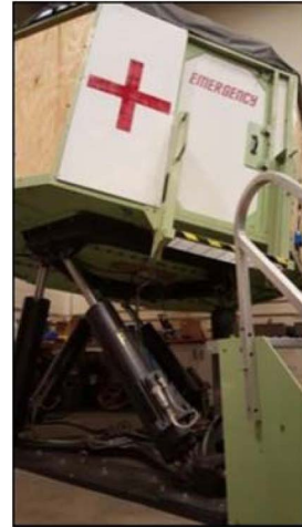
FIGURE 1. Simulator used in this study: Moog Series 6DOF500E, Model 170.
