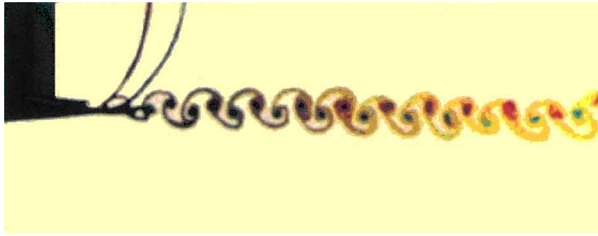
Fig. 2 Vortex patterns for a stationary NACA 0012 airfoil for a freestream velocity of 0.2 m/s.
