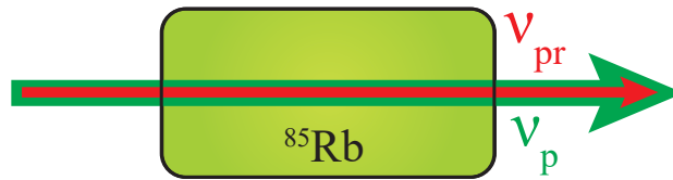
Figure 4.3. Laser alignment through Rb cell for the EIT experiment.
