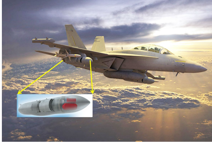
Figure 10. NGJ-MB On Board the EA-18G Growler. Source: DOT&E (2020).
