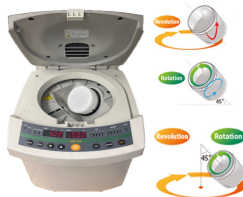
Figure 3.7. The Planetary centrifuge both rotates the mixture about the central axis of the machine and rotates the container at a 45 degree angle. This process ensures uniform mixing. Source: [18]
