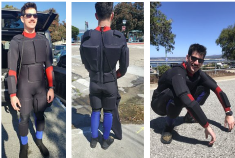
Figure 4.1. Pictured are the front of the suit (left), the back of the suit (middle), and a squatting position to show the suit's range of motion (right). The thin sections at the joints allowed for full arm and shoulder rotation, much like a surfing wetsuit. The composite wetsuit was noticeable heavier than the neoprene wetsuit, but about five extra pounds were needed to counter the added buoyancy of the composite paneling.
