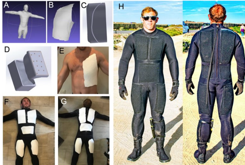
Figure 2.10. (A) A full body scan rendered the geometry to be approximated for individual casting (B) Areas of the scan were cut into individual pieces to be cast (C/D) The curved positive geometry was then converted into a mold (E) The HGM composite was cast in each body curve shape (F/G) All finished pieces were laid out on a thin custom neoprene wetsuit. (H) The composite material was attached to the suit in thinner neoprene pockets. The full suit was field tested. Source: [19]
