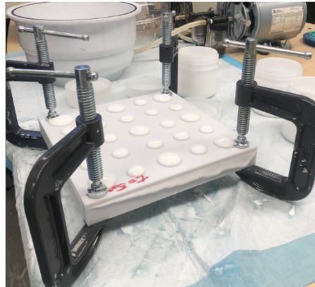
Figure 4.7. The clamped assembly secured the lid in place as the composite cured in the sample size molds.
