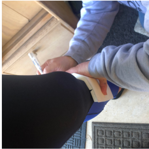
Figure 3.11. A composite piece is laid out on the thigh and traced by a custom wetsuit tailor.
