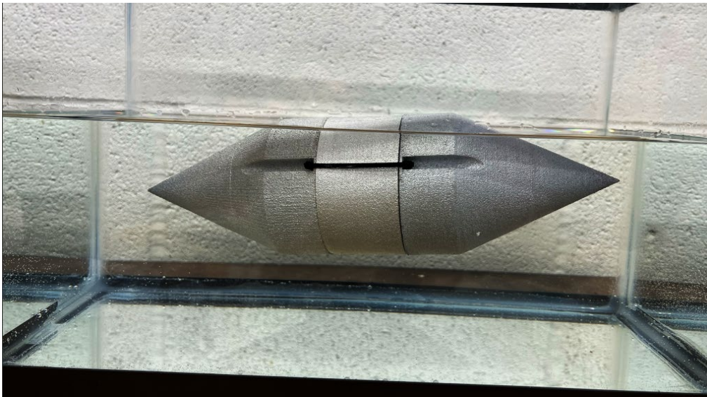
Figure 54. Assembly 23 During Payload v2 Test (Using Configuration 2 – 1.5 mm Walls)
