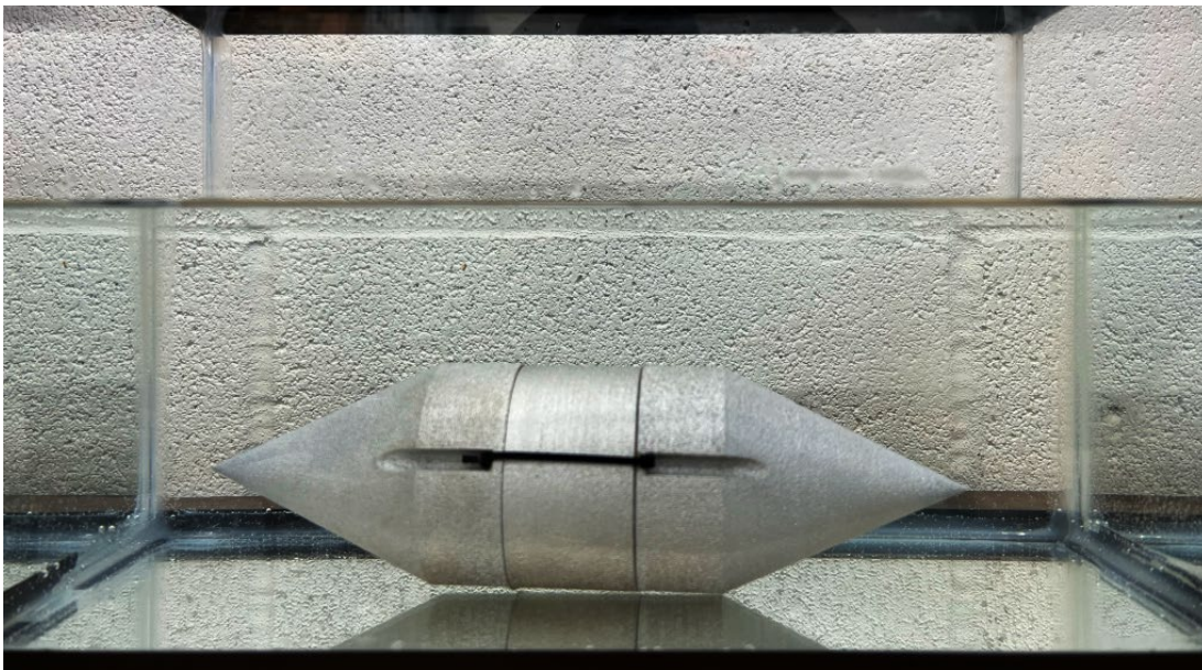
Figure 56. Assembly 30 During Payload v2 Test (Using Configuration 3 – 2 mm Walls)
