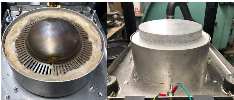
Figure 23. Heat Shield Insulation (left) and Assembly (right).
