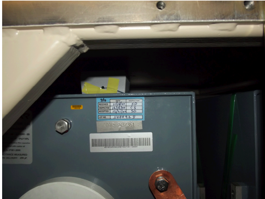
Figure 21 – This photograph shows the wireless Bluetooth tag inside protective plastic box, with full sensor suite sitting on upper surface of 22-kV 22-kJ capacitor during charge-discharge testing in LLNL Building 291 basement (pulsed power laboratory).
