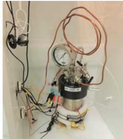
Argon-filled autoclave with copper tubing and electronic connections
