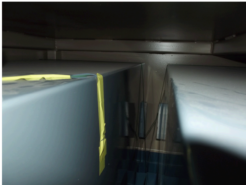
Figure 22 – This photograph shows fiber optic strain gauge being used as independent verification of wireless strain gauges; the wireless strain gauges have not yet been glued down to capacitor surface. Initial tests were designed to demonstrate data transmission in such high-energy high-field environments, relevant for grid storage applications.
