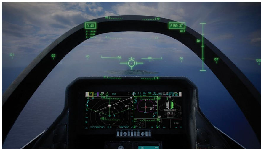
Figure 8. Point of View (Simulated) Using F-35 HMD Helmet. Source: Navy's F-35 Helmet Problem Fixed With TV Technology (n.d.).
