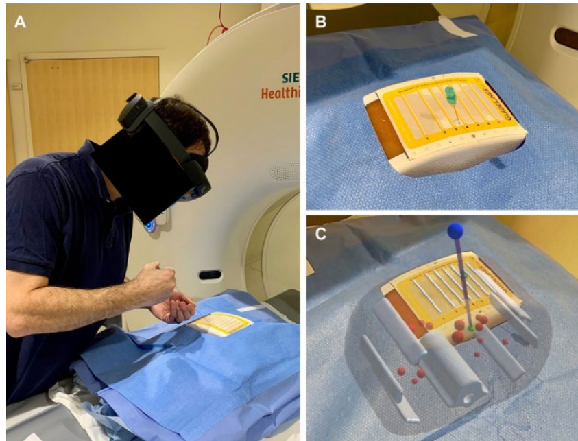
Figure 6. AR-Assisted Navigation Using HoloLens 2. (A) Participant performing the medical procedure while wearing a HoloLens 2. (B) Control image of needle insertion without AR. (C) View through HoloLens 2 of needle insertion with virtual needle guide and three-dimensional phantom model projected onto the true phantom. Source: Park et al. (2020).
