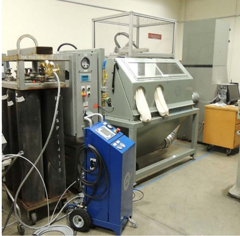
Figure 8. Centerline SST Model Series C low-pressure cold spray system installed at the Naval Postgraduate School.
