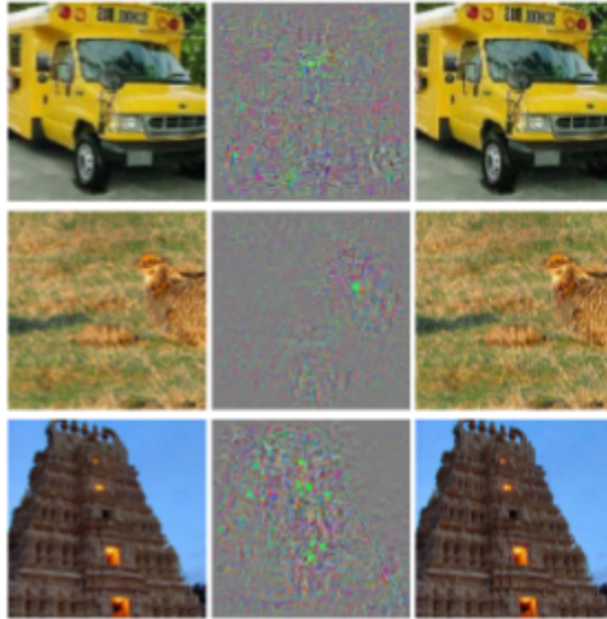
Figure 2.2. Left shows the original input, middle shows the perturbations that are added to the photo on the left, and right shows the resulting adversarial example image. The images on the left are correctly classified, and the images on the right are misclassified as an ostrich, struthio, and camelus. Source: [15].
