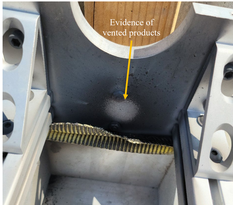
Figure 29. Test stand head-end after live-fire test
