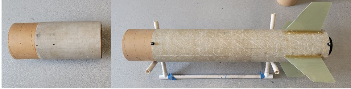
Figure 56. First stage booster (right) and parachute bay (left)
