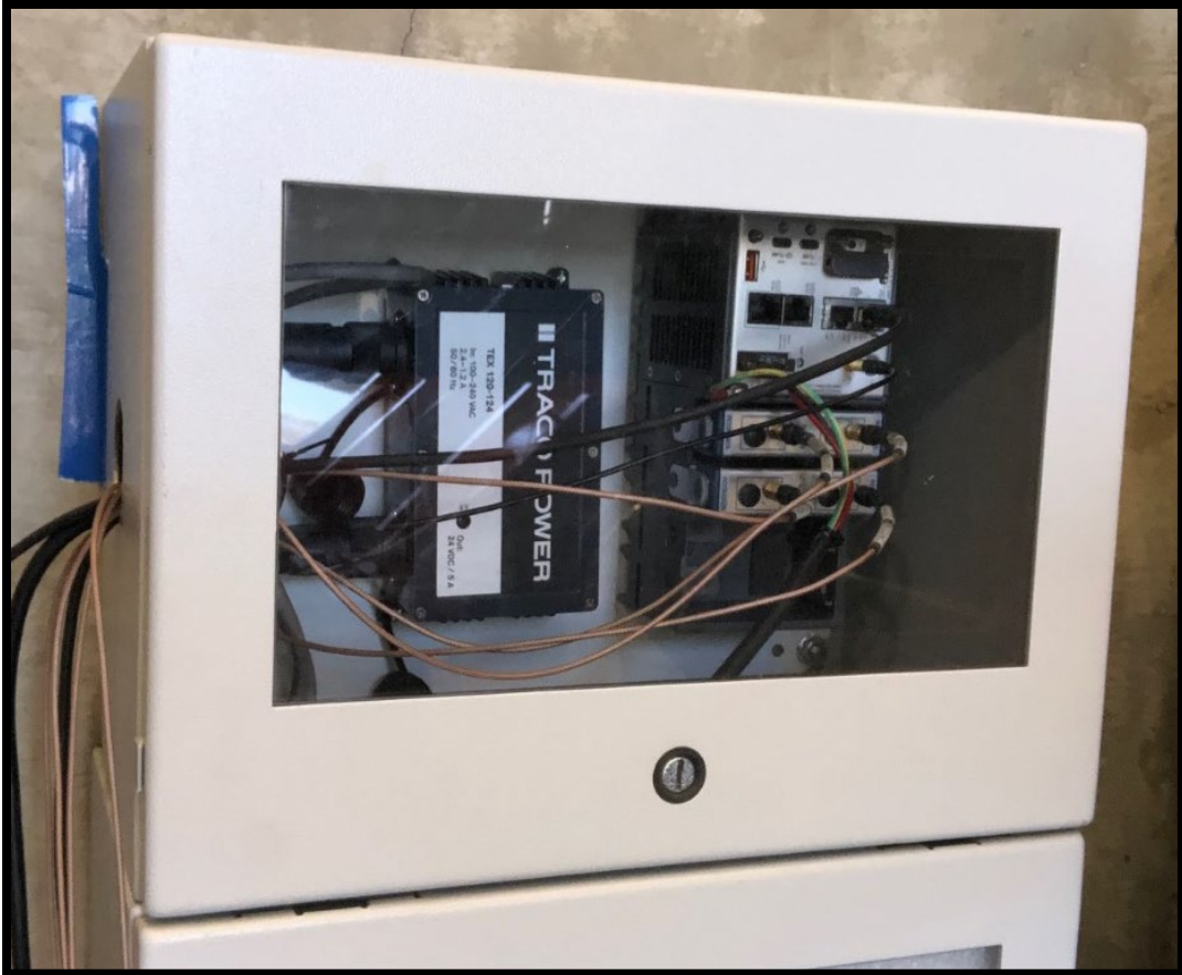
Figure 112. Casing for Data Acquisition Used on BCTR (Tip Gap Casing) and TCR Experiments.
