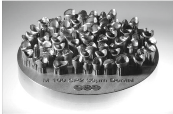
Fig. 6.51 Example of AM CoCr dental crowns (Schweiger et al. [71], 2010.—licensed under CC BY 4.0)
