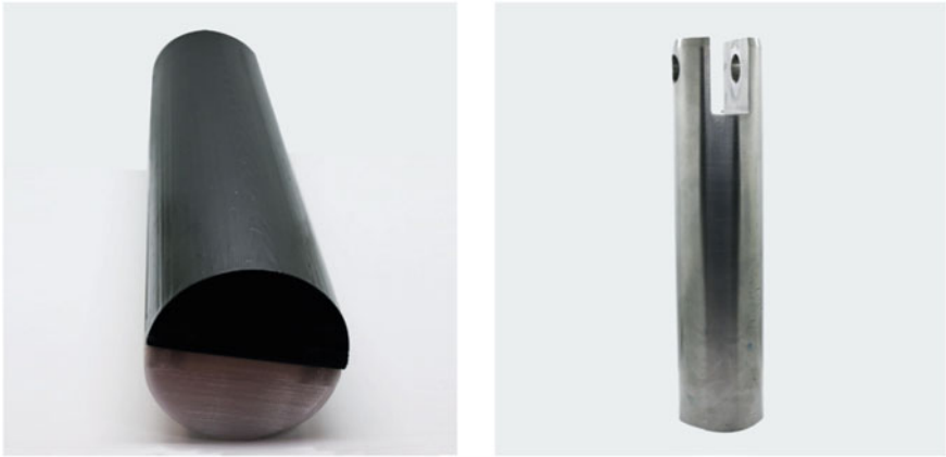
Fig. 6.79 Left: 3D pattern (bottom)/wood pattern (top). Right: Guide bar (Courtesy of Wilhelmsen group and Ivaldi group)
