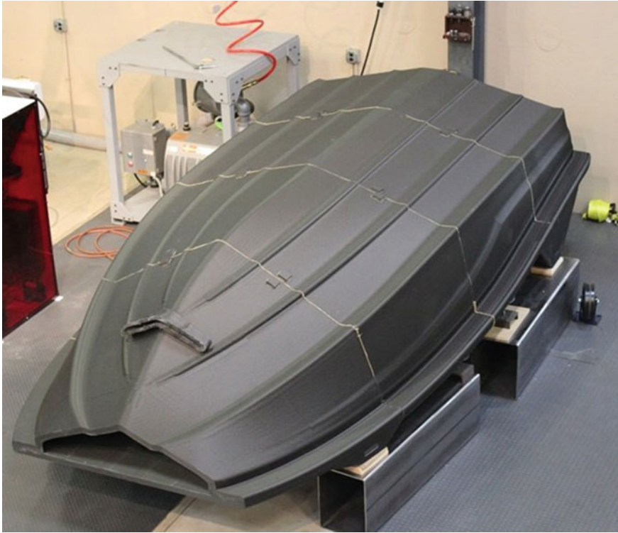
Fig. 6.82 Boat hull pattern after bonding together and before machining (Courtesy of Thermwood)
