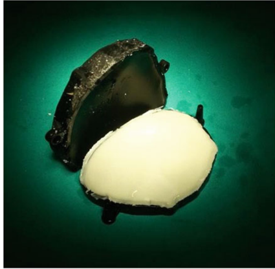
Fig. 6.60 Example of AM (PolyJet) mould for production of bone cement cranial implant ( Source AdTec SME project—UNIZAG FSB)
